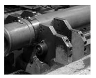
Prior to fitting, alignment/offset between the two end fittings is performed. The phase tolerance between the two end fittings is  $\pm 20$ . The offset of both components (shaft and end fitting) is always checked, in automatic, at the end of each work cycle.
