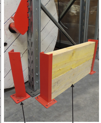
Ladder foot protection
