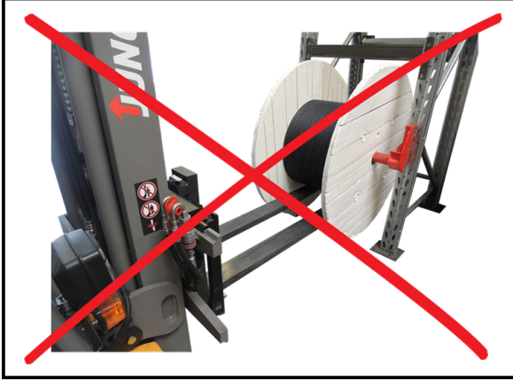
The cable drum at risk of falling. The cable may be damaged.
