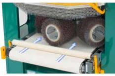
The strong, compact gear head is equipped with a total of six spindles, mounted in pairs, rotating alternately clockwise and counterclockwise.
